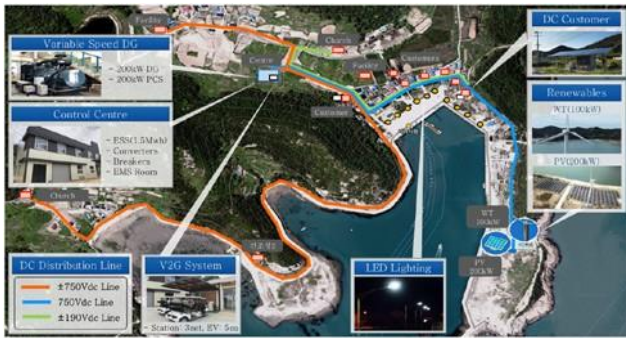
Fig. 2 Equipment and network configuration of DC Island
